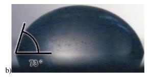
Fig. 13 Photos of the progressive contact angles: a) Polyurethane coated non-electro-polished sheet with a 30 μl drop, b) Polyurethane coated electro-polished sheet with a 30 μl drop
