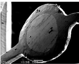
Fig. 4 Radiopaque platinum marker of Tecnic Carbostent<sup>TM</sup> at 130 times magnification
