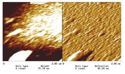
Fig. 5 Atomic force microscopy image of Tecnic Carbostent<sup>TM</sup>
