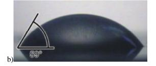
Fig. 14 Photos of the receding contact angles: a) Polyurethane coated non-electro-polished sheet with a 30 µl drop, b) Polyurethane coated electro-polished sheet with a 30 µl drop
