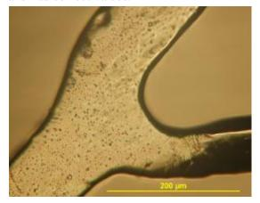
Fig. 1 Smooth surface of Tecnic Carbostent<sup>TM</sup>, after expansion at 200 times magnification
