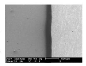
Fig. 6 Smooth polyurethane coating on sheet at 39 times magnification
