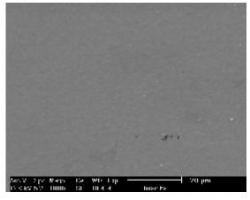
Fig. 10 Smooth texture of the sheet after having been dipped five times into 1w/w% tetrahydrofuran solution at 1000 times magnification
