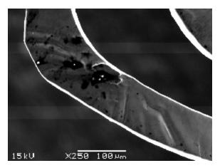
Fig. 3 Fragment resulting from cutting after expansion of Tecnic Carbostent<sup>TM</sup> at 250 times magnification
