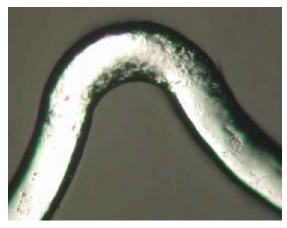
Fig. 2 Strain-lines of Tecnic Carbostent<sup>TM</sup>, after expansion at 200 times magnification
