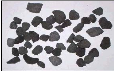
Fig. 5, Loose glass foam
