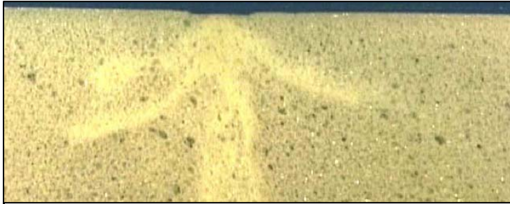
Fig. 9, Polyurethane foam with local foam collapse
